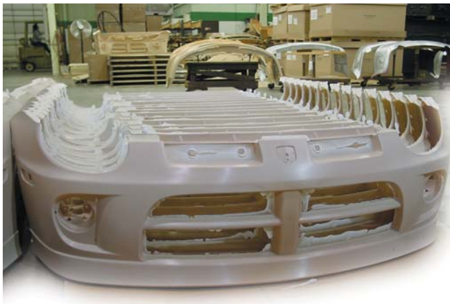
The end product of the molds shown: automotive fascias ready to be deburred and shipped.
